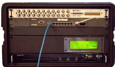
Figure 2 Node computer in SYSLAB
