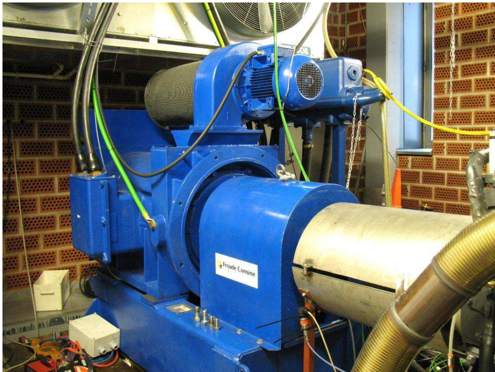
The diesel-motor dynamometer can be used to emulate the primary energy source.
