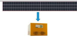
Three double strings could directly feed into three MPPT inputs of one MSXI-3336 inverter module. A 500kW MODGES POWER STATION consists of 16 MSXI-3336 modules and 48 MPPT inputs.
