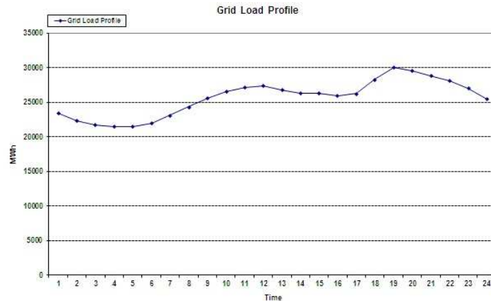
Fig.2. Load profile of grid in 24 hours duration
